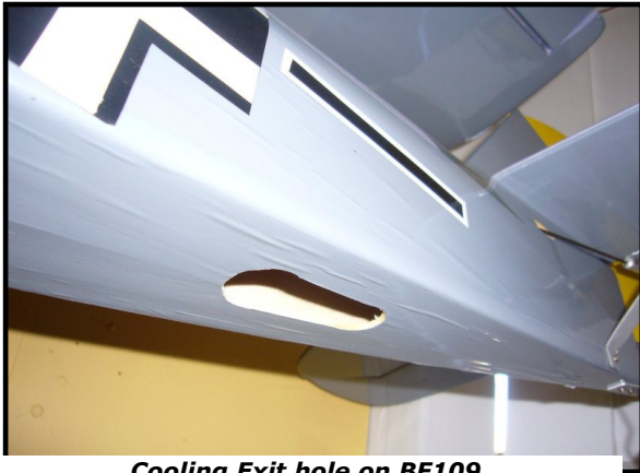
Cooling Exit hole on BF109
